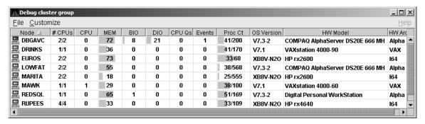
Within each group of nodes displayed, the Availability Manager displays all the nodes with which it can communicate. If some nodes in the group are not displayed, it is because the Availability Manager has not received a multicast "Hello" message from the Data Collector on that node.
