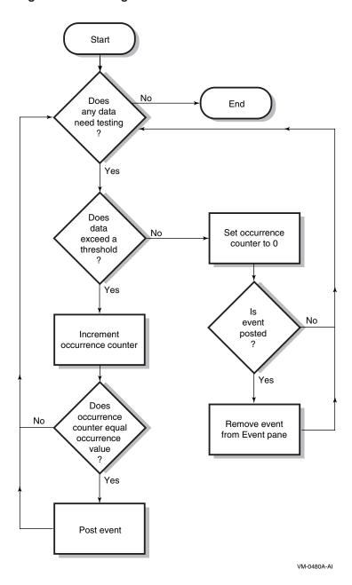
Figure 5-3 Testing for Events
