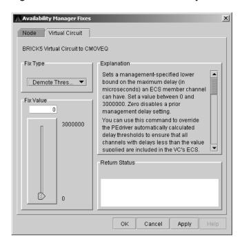
Figure 6-26 LAN VC ECS Maximum Delay
