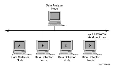
In Figure 1–2, the Data Analyzer can monitor nodes A, B, and C across the network. The password on node D does not match the password of the Data Analyzer; therefore, the Data Analyzer cannot monitor node D.
