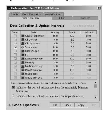
Figure 7-6 OpenVMS Operating System Customization
