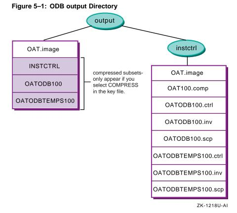
The subset files and the files in the instctrl directory are constituents of the final kit. The following sections describe the contents of the installation control files created by the kits utility.
