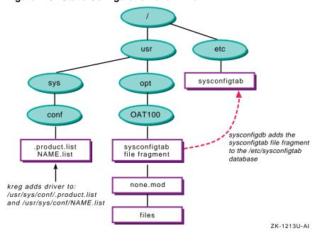
Figure 7-5: Static Configuration of a Driver
